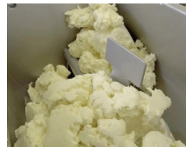
View at the end of mixing before emptying the butter
